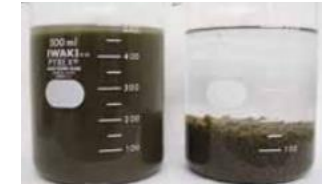
Hakuto's proprietary wastewater treatment chemical "HAKUTORON" is used in the primary treatment of contaminated water, improving the operational efficiency of distillation equipment (from left to right: before and after treatment).
